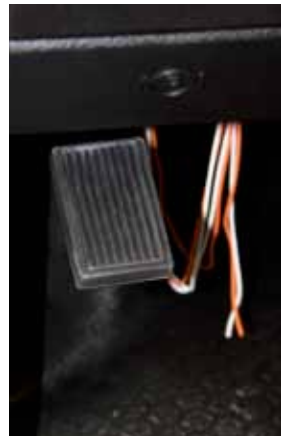
Flasher Activation Wires
