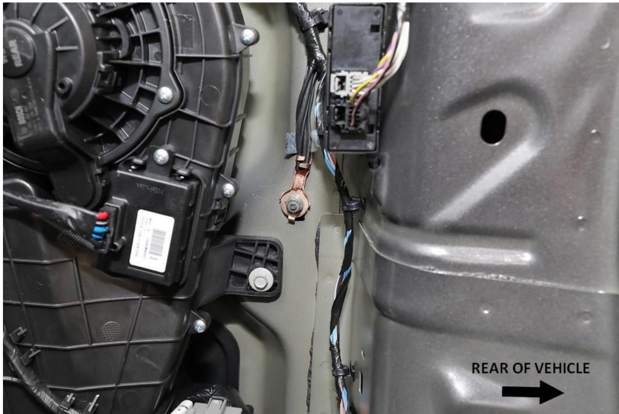
Figure 13: Passenger's Side D-Pillar Ground Location (Driver's Side Similar)
