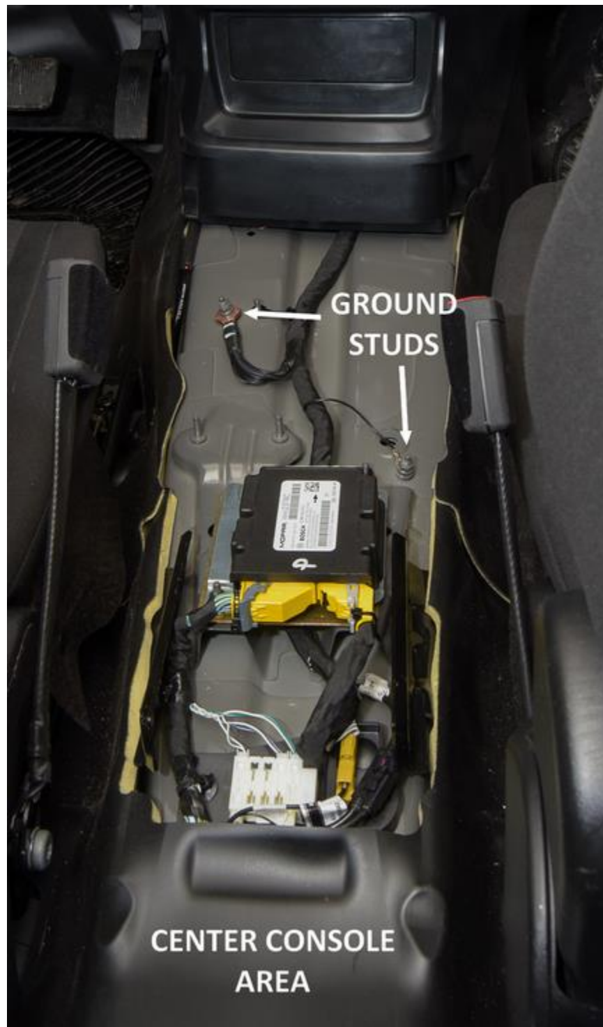
Figure 11: Center Console Grounding Locations
