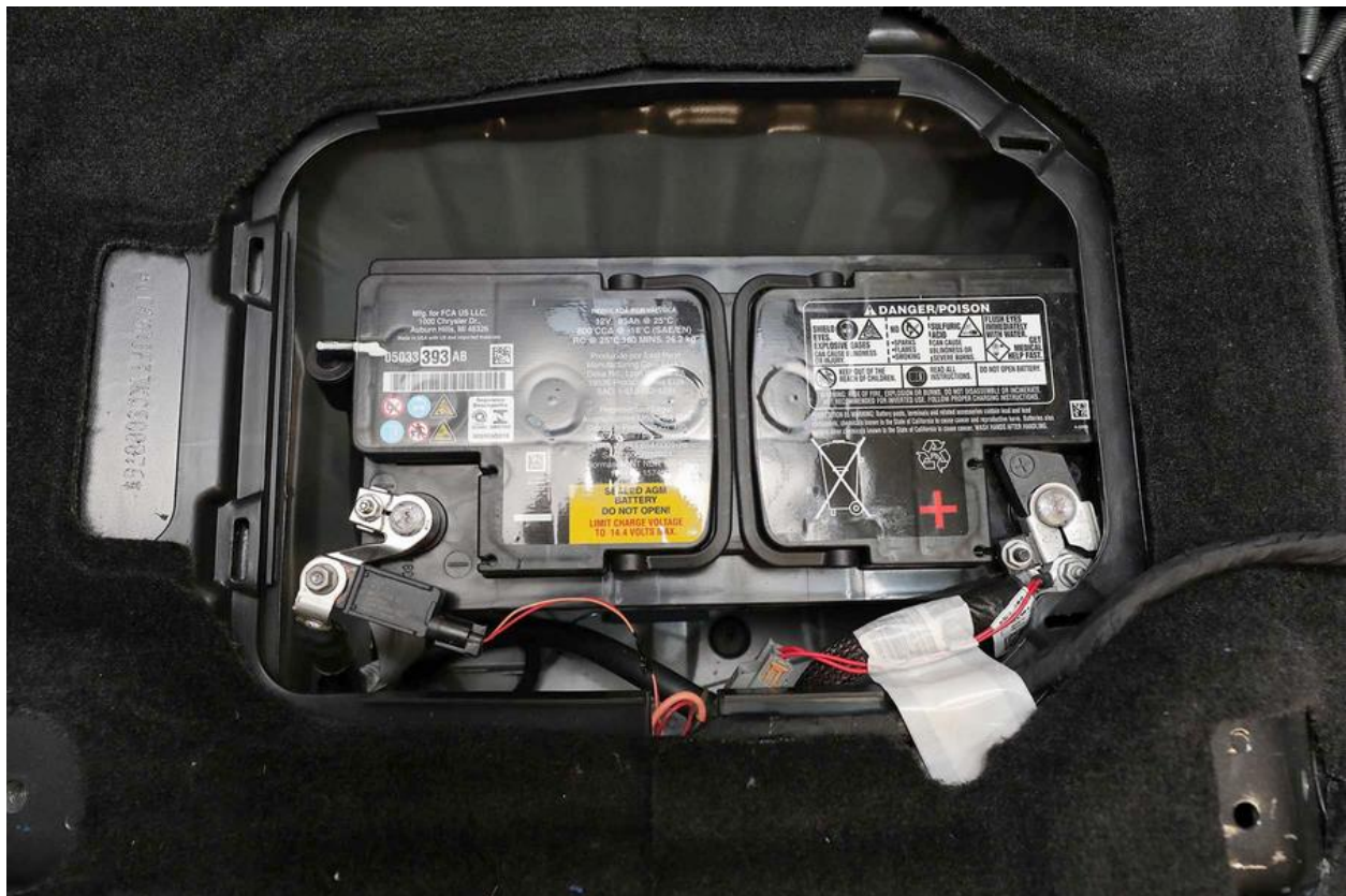
Figure 8: Battery Under Passenger Seat (V8 model shown)
